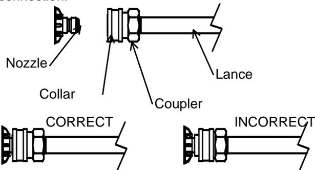
**WARNING:** Make sure the nozzle is correctly inserted. The nozzle may become a projectile if not inserted correctly. Do not attempt to use different types of nozzles that may not fit the coupler.
