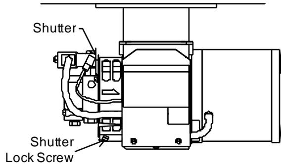
***CAUTION: If white smoke appears from the burner exhaust vent during start-up or operation, discontinue use and readjust air bands.***
