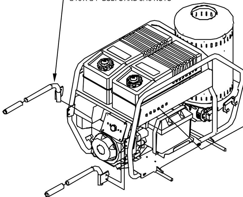
INSTALL GROMMETS AND NOZZLES INTO HOLES IN FRAME
