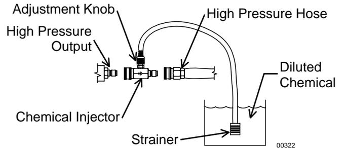
B.) You need to use the low pressure nozzle to spray chemicals onto the cleaning surface.
