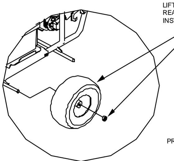
LIFT BACK OF UNIT BY HANDLES TO INSTAL ALL REAR WHEELS, THEN LIFT FRONT OF UNIT TO INSTAL FRONT WHEELS
