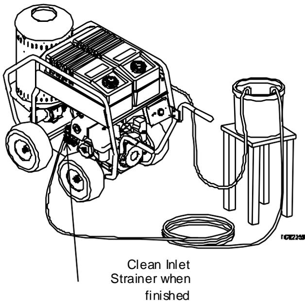
6. Run the pressure washer in cold mode for 1 to 3 hours re-circulating the cleaning solution.
