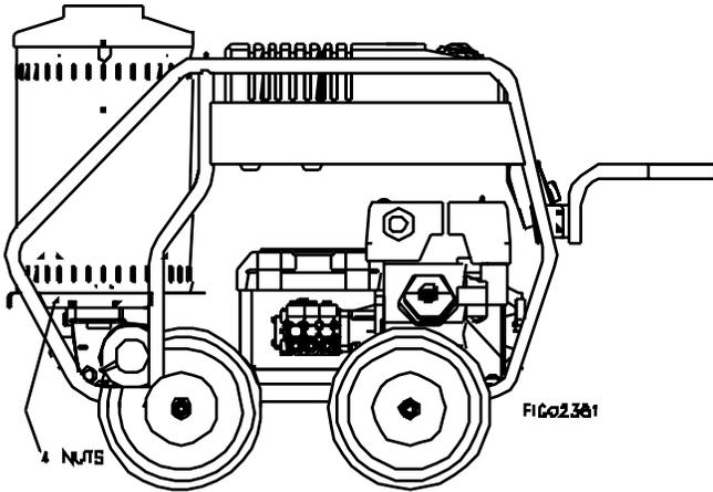
2. Pull the burner out from underneath the heat exchanger. Tip the burner away from the machine so the electrodes are visible.
