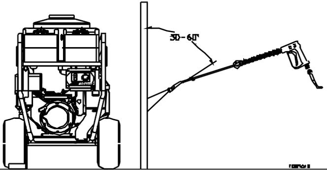
It is recommended that a partition be made between the wash area and the pressure washer to prevent direct nozzle spray from coming in contact with the pressure washer. Moisture reaching the equipment will reduce the pressure washer's service life.
